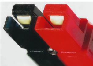
Anderson Power Poles are universal connectors that are often used so that components can be interchanged with other systems. Soldering these connections works better than crimping. Make sure the polarity is correct - Red on the right and metal pin on top.
