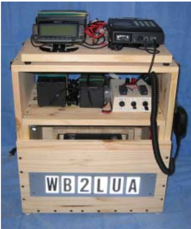
Battery Module with Radio Equipment on top
