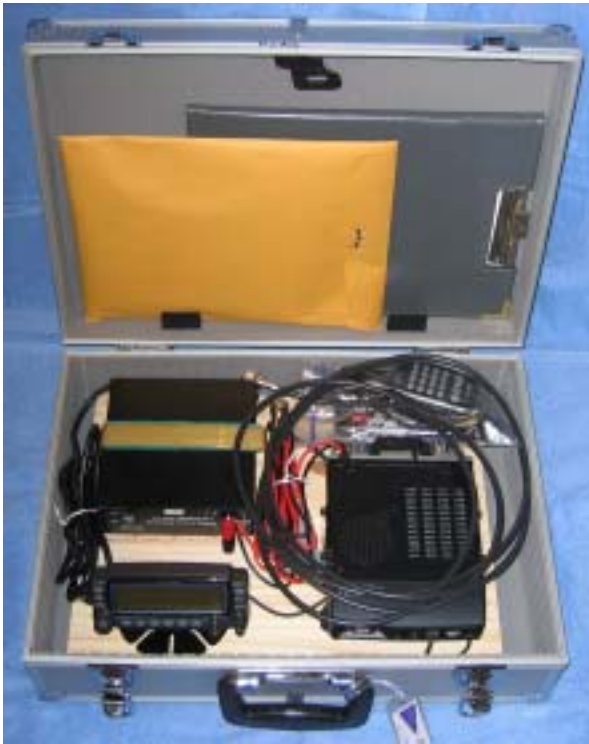
Case 1 (Radio, AC Power Supply mounted on a board)
