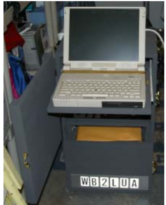
The notebook computer is mounted on a double sliding shelf system. The computer shelf height is 26.75", which is good for typing. This height determined the total height of the station.
