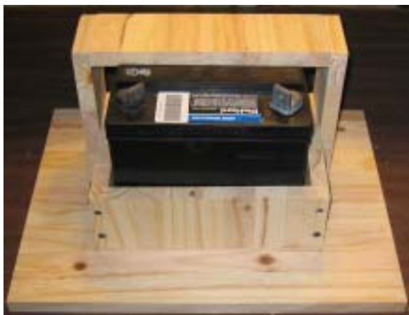
Battery Mounting (bracketed to the bottom)
